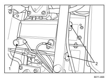
1. Terminal guard 2. Battery hold downs *Battery installation*
